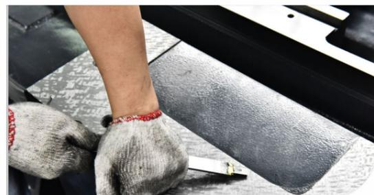
■ All joint surfaces of the machine body through manual scraping to ensure geometric accuracy and contact surface rigidity.
