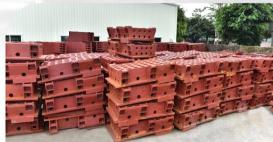
■ The machine body adopts high strength HT300 gray casting iron through more than six months of aging treatment after high temperature tempering, which could eliminate the internal stress by maximum.
