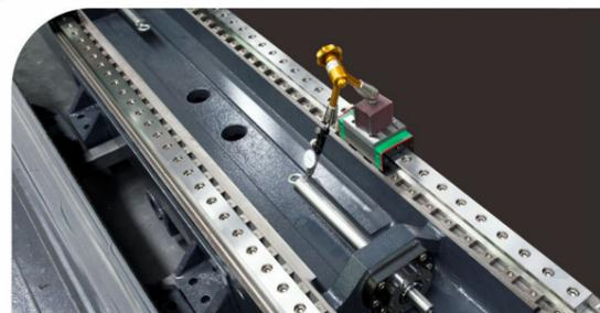
■ Adopt Japanese NSK/THK ball screw, assembled by experienced engineer, strictly control the straightness of the screw nut.
