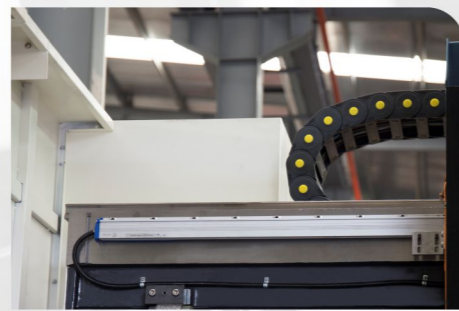
Linear scale 3 axis with optional fully closed loop inspection system
