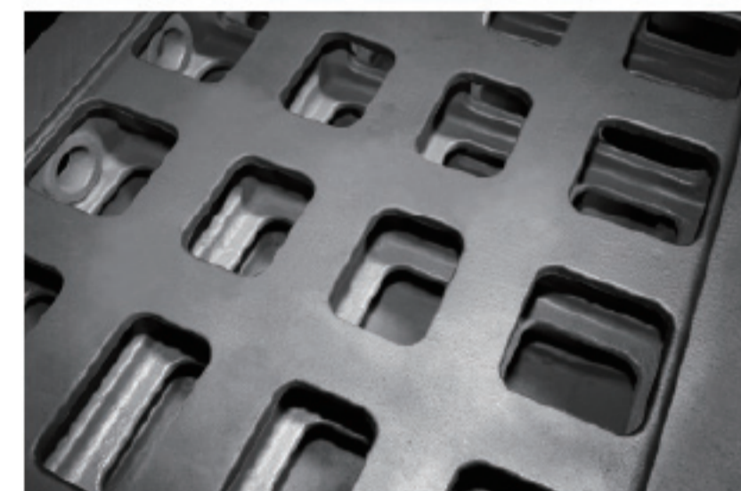
Base, worktable, and gantry beam all adopt a box-shaped double-layer rib structure;
