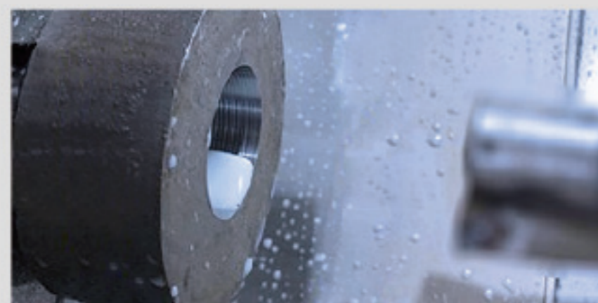
U Drill punch hole processing
