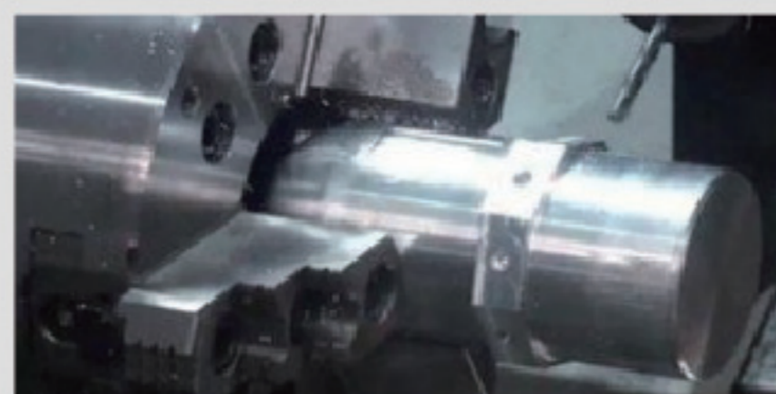
Circumference drilling & tapping
